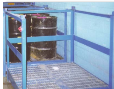
Example of using racks to protect drums from physical damage from traffic.
