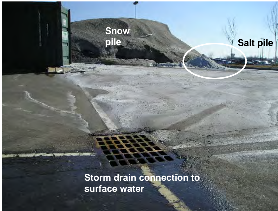
Figure 6. Incorrect Salt Storage: uncovered and placed in path of melting snow pile
