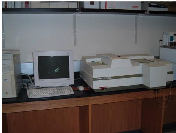
Figure 4: UV-VIS Spectrophotometer
