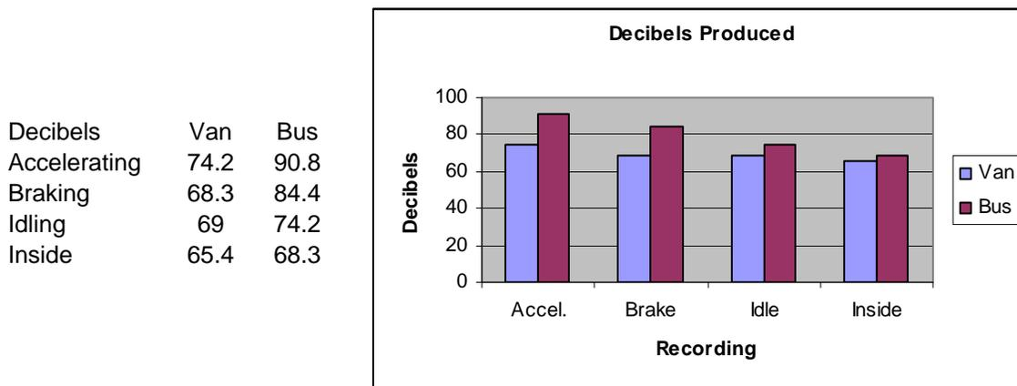
Chart 1 and Figure 1: Decibel levels recorded during different parts of a vehicle’s route.
