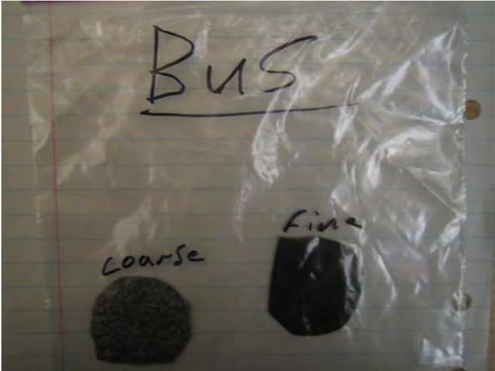
A clear difference between the vehicles can be seen with the naked eye. While the van filter appeared virtually identical before and after the test, the bus filter had turned almost black after 1 minute of exhaust filtration. The filter samples were taken back to the lab for microscopic analysis.
