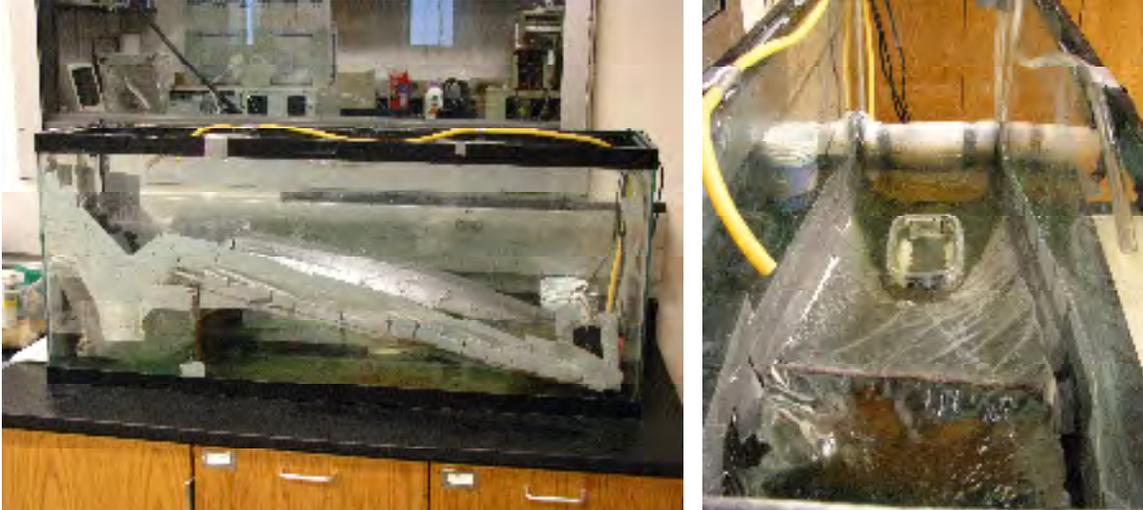
Fig.6. In-lab stream simulator
