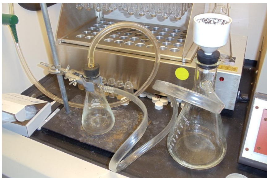
Figure 1: Vacuum filtration set up using 7 micron glass fiber filters.
