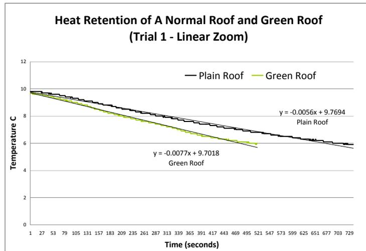
Figure 6. Trial 1. This graph shows how temperature decreases with time. The green roof releases heat at a slightly faster rate than the plain roof, which was not what was expected. The linear portion of Trial 1 was zoomed in on, and a linear trend line was fit to the data points.
