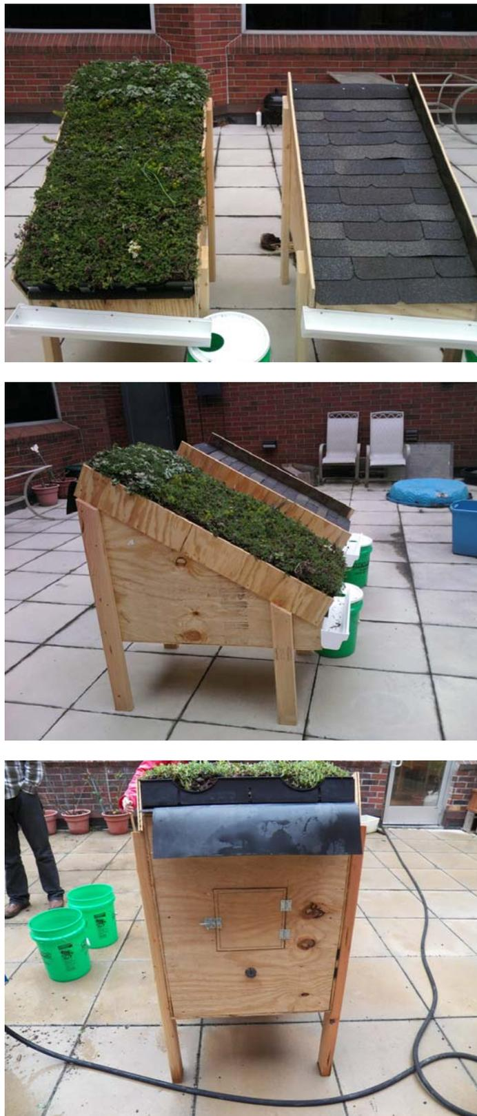
Figure 1: Front, side, and back views of the constructed roof models
