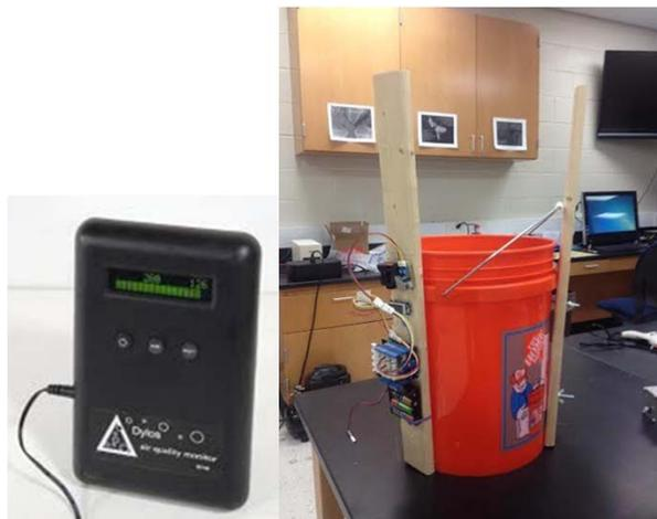
Figure 5: Devices that can be used in residential homes to sample air quality
