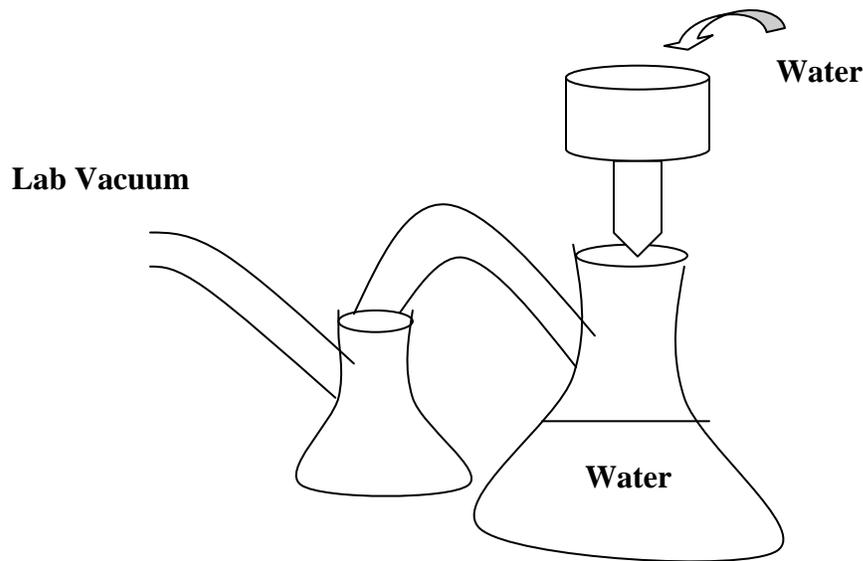
Figure 1: Vacuum filtration set-up
