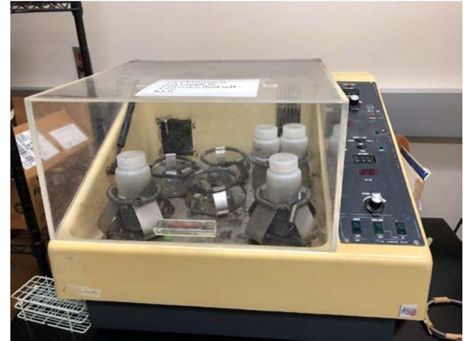
An image of the shaking machine used to agitate our samples and promote leaching
